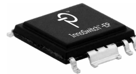
Figure 2. High Creepage, Safety-Compliant eSOP-R16B Package.
