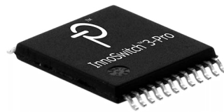
Figure 2. High Creepage, Safety-Compliant InSOP-24D Package.
