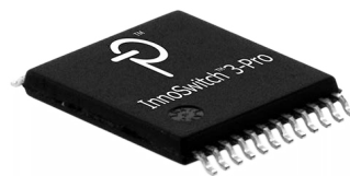
Figure 2. High Creepage, Safety-Compliant InSOP-24D Package.
