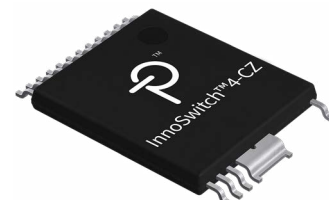
Figure 2. High Creepage, Safety-Compliant InSOP-24D Package.
