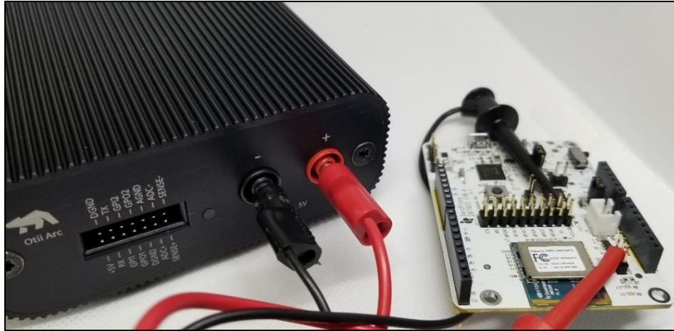
Figure 14: Current measurement setup using Otti Arc
