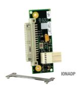
The IONADP is an adapter card that allows the ION Platform chassis to be backwards compatible with Point System<sup>™</sup> modules. This adapter is designed to sit between a Point System<sup>™</sup> module and the backplane of the ION chassis. The purpose of the IONADP is to lengthen the Point System<sup>™</sup> module so it can be securely mounted in an ION chassis while also connecting to the backplane allowing the ION chassis to power the Point System<sup>™</sup> module.
