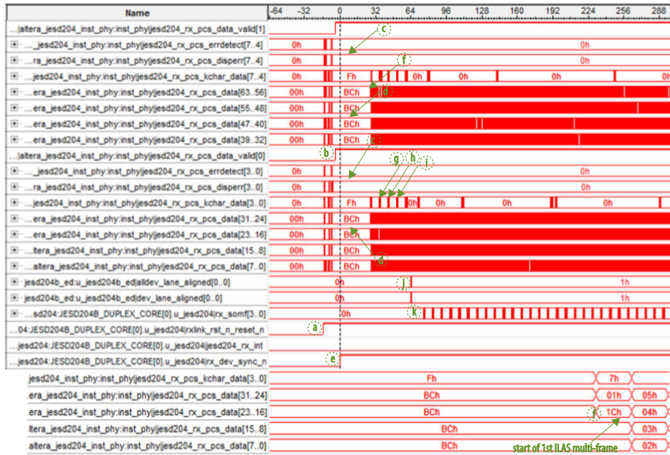
Figure 33. JESD204B Link Initialization
