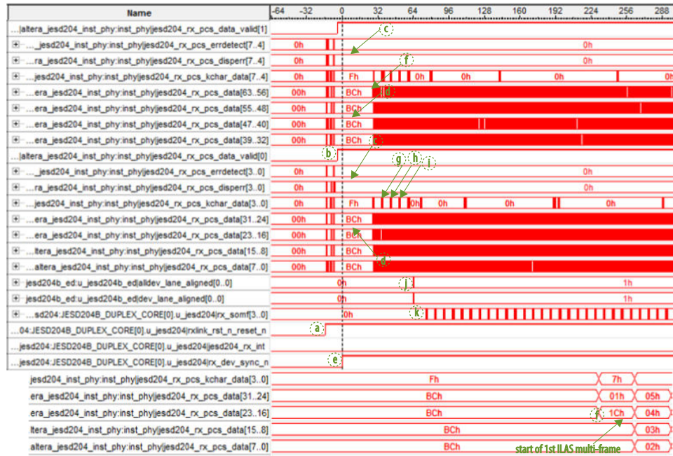
Figure 34. JESD204B Link Initialization
