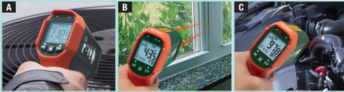
A. HVAC/R Diagnostics - Diagnose ventilation systems outdoors in rain or shine conditions B. Insulation Inspection - Blue LED flashes when temperature is below low alarm set point C. Automotive troubleshooting - Red LED flashes when temperature is above high alarm set point
