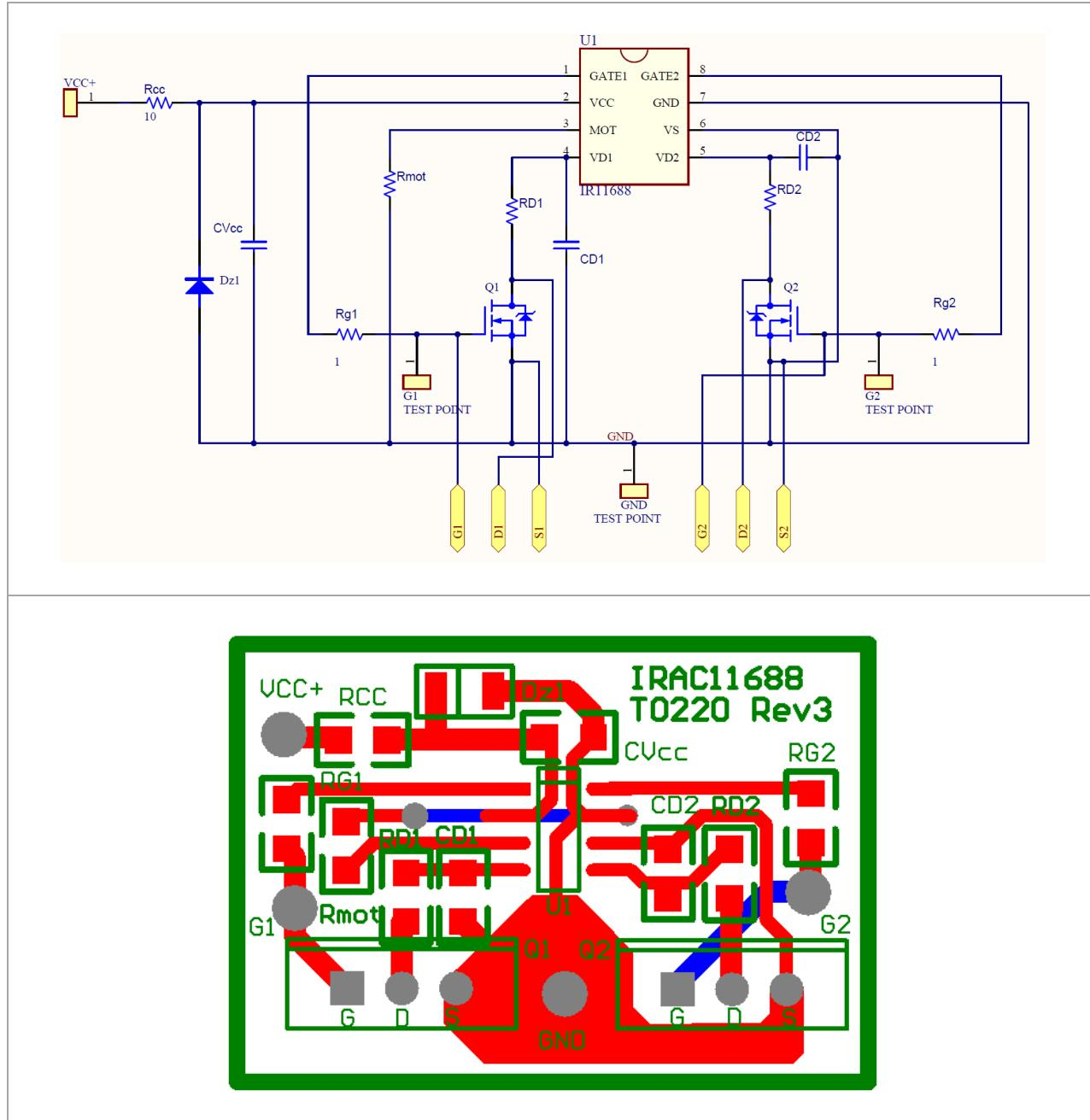
The daughter card shown above is designed to allow easy retrofit in existing systems with minimal system changes. The component values are recommended but user has freedom to change them per application requirement.
