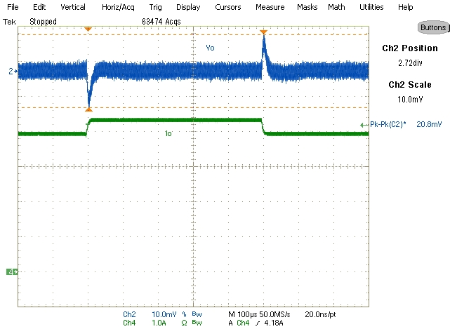
Transient response-Sourcing mode Vin-1.5V Vout-0.75V/3.9-4.3-3.9A Ch4-Vout Ch3-Iout (1A/ \mu Sec slew rate)
