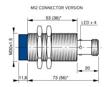
(\*) The dimensions in brackets refer to short housing models Note: the front part in blue is valid only for unshielded models
