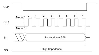
Figure 8.129 Write PPB Lock Bit Sequence In QPI Mode
