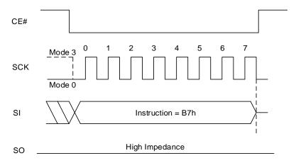
Figure 8.107 Enter 4-byte Address Mode Sequence In QPI Mode
