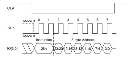
Figure 8.99 Sector Unlock Sequence In QPI Mode (26h [EXTADD=1] or 25h, 4-byte address)
