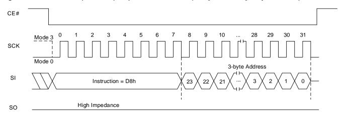
Figure 8.32 Block Erase (64K/256K) Sequence In SPI Mode (D8h [EXTADD=1] or DCh, 4-byte address)
