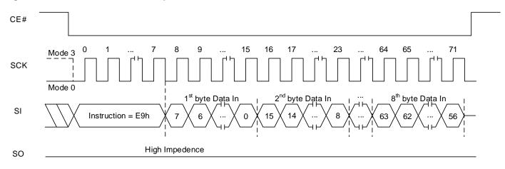
Figure 8.137 Unlock Password Sequence In QPI Mode
