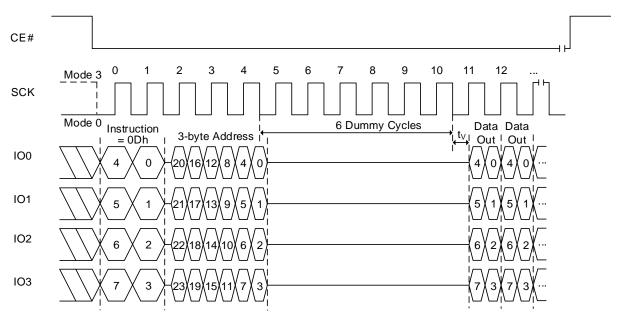
Figure 8.84 FRDTR Sequence In QPI Mode (0Dh [EXTADD=0], 3-byte address)
