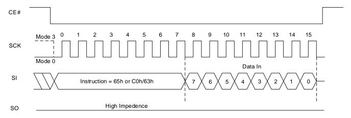
Figure 8.60 Set Read Parameters Sequence In QPI Mode
