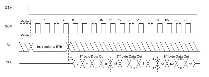
Figure 8.133 Read Password Sequence In QPI Mode
