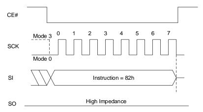
Figure 8.68 Clear Extended Read Register Sequence In QPI Mode
