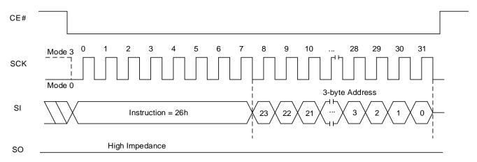
Figure 8.97 Sector Unlock Sequence In SPI Mode (26h [EXTADD=1] or 25h, 4-byte address)
