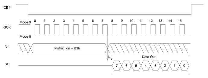
Figure 8.153 Read ECC Register In QPI Mode
