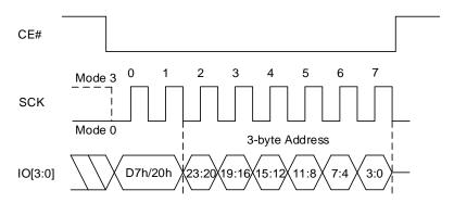
Figure 8.30 Sector Erase Sequence In QPI Mode (D7h/20h [EXTADD=1] or 21h, 4-byte address)
