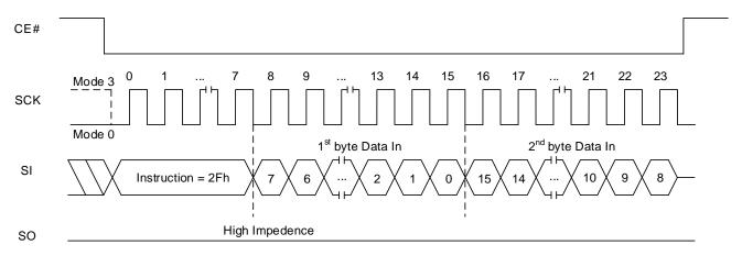
Figure 8.126 Program ASP Sequence In QPI Mode
