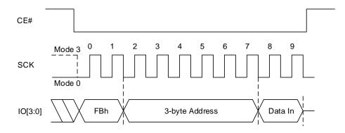
Figure 8.115 Write DYB Sequence In QPI Mode (FBh [EXTADD=1] or E1h, 4-byte address)
