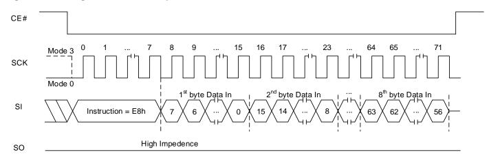
Figure 8.135 Program Password Sequence In QPI Mode
