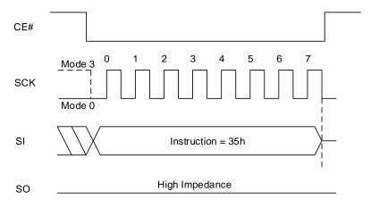
Figure 8.54 Exit Quad Peripheral Interface (QPI) Mode Sequence
