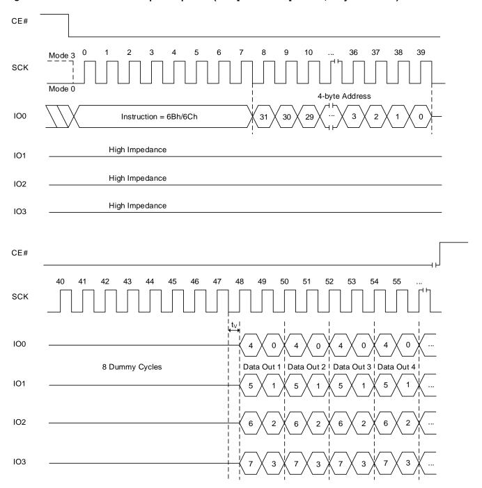
Note: Dummy cycles depends on Read Parameter setting. Detailed information in Table 6.11 Read Dummy Cycles.
