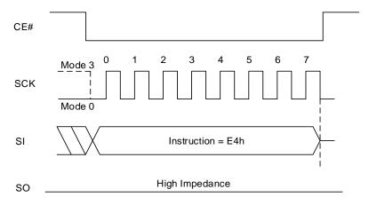
Figure 8.123 Erase PPB Sequence In QPI Mode
