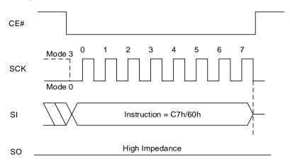
Figure 8.40 Chip Erase Sequence In QPI Mode
