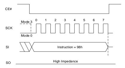
Figure 8.141 Gang Sector/Block Unlock Sequence In QPI Mode
