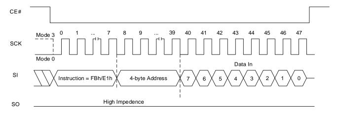
Figure 8.114 Write DYB Sequence In QPI Mode (FBh [EXTADD=0], 3-byte address)
