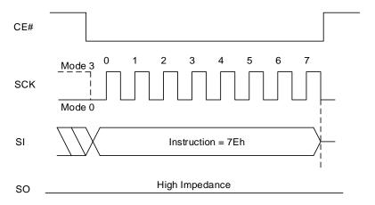
Figure 8.139 Gang Sector/Block Lock Sequence In QPI Mode
