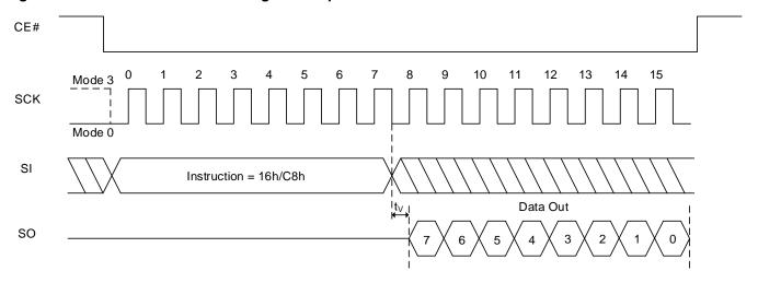
Figure 8.103 Read Bank Address Register Sequence In QPI Mode
