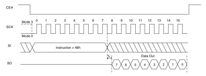
Figure 8.50 Read Function Register QPI Sequence
