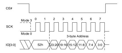
Figure 8.38 Block Erase (32K) Sequence In QPI Mode (52h [EXTADD=1] or 5Ch, 4-byte address)
