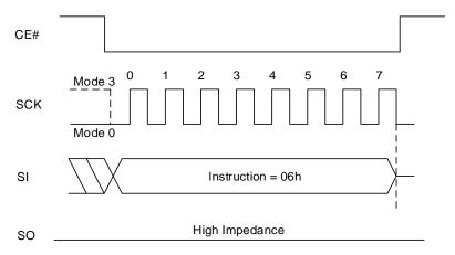
Figure 8.42 Write Enable Sequence In QPI Mode
