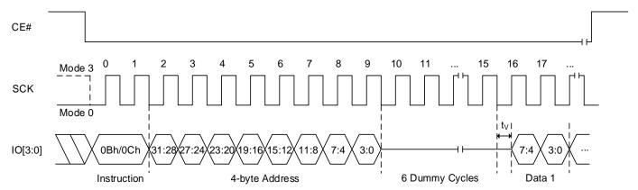
Note: Number of dummy cycles depends on Read Parameter setting. Detailed information in Table 6.11 Read Dummy Cycles.
