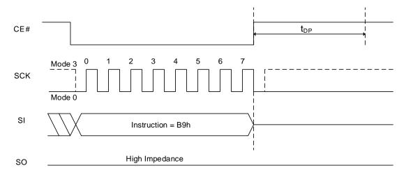
Figure 8.56 Enter Deep Power Down Mode Sequence In QPI Mode
