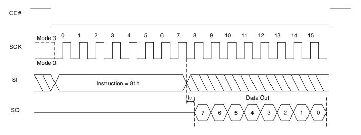
Figure 8.66 Read Extended Read Parameters Sequence In QPI Mode
