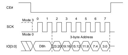
Figure 8.34 Block Erase (64K/256K) Sequence In QPI Mode (D8h [EXTADD=1] or DCh, 4-byte address)
