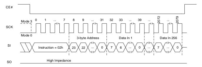
Figure 8.22 Page Program Sequence In QPI Mode (02h [EXTADD=0], 3-byte address)
