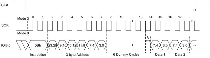
Note: Number of dummy cycles depends on Read Parameter setting. Detailed information in Table 6.11 Read Dummy Cycles.
