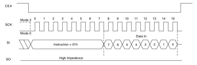
Figure 8.48 Write Status Register QPI Sequence
