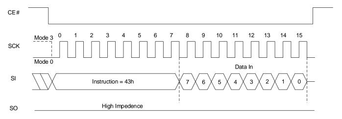
Figure 8.145 PNVDLR Sequence In QPI Mode
