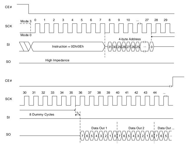
Note: Dummy cycles depends on Read Parameter setting. Detailed information in Table 6.11 Read Dummy Cycles.
