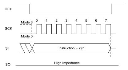
Figure 8.109 Exit 4-byte Address Mode Sequence In QPI Mode
