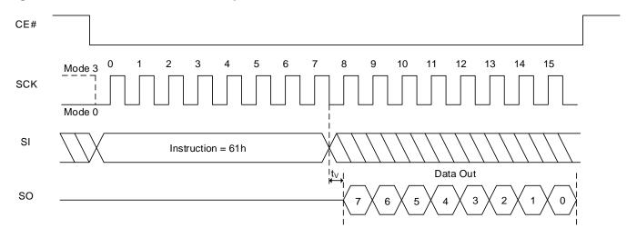
Figure 8.64 Read Read Parameters Sequence In QPI Mode
