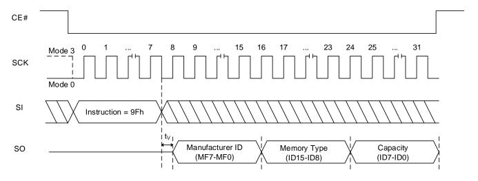
Figure 8.72 RDJDID and RDJDIDQ (Read JEDEC ID) Sequence In QPI Mode
