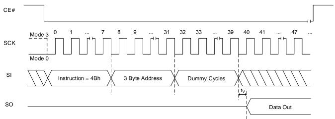
Note: Dummy cycles depends on Read Parameter setting. Detailed information in Table 6.11 Read Dummy Cycles.
