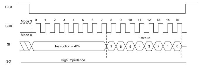
Figure 8.52 Write Function Register QPI Sequence
