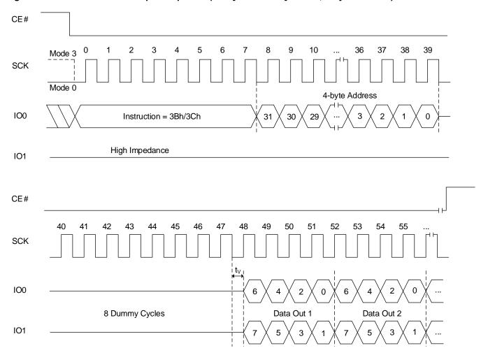
Note: Dummy cycles depends on Read Parameter setting. Detailed information in Table 6.11 Read Dummy Cycles.
