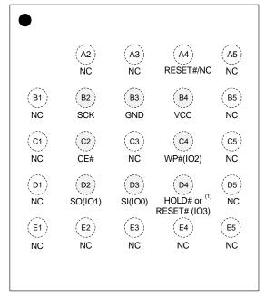
24-ball LFBGA 6x8x1.40mm (5x5 ball array) (Package: I)
