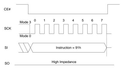
Figure 8.131 Set FREEZE Bit Sequence In QPI Mode
