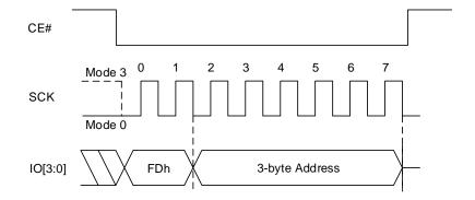
Figure 8.121 Program PPB Sequence In QPI Mode (FDh [EXTADD=1] or E3h, 4-byte address)
