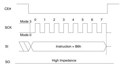
Figure 8.155 Clear ECC Register Sequence In QPI Mode
