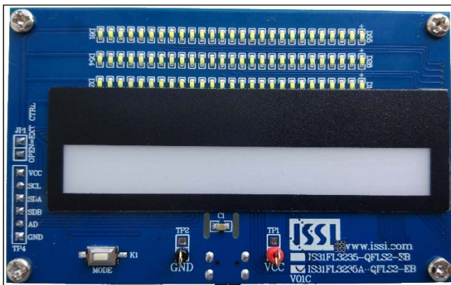
Figure 8: Photo of IS31FL3235A Evaluation Board (LPC922 Version)
