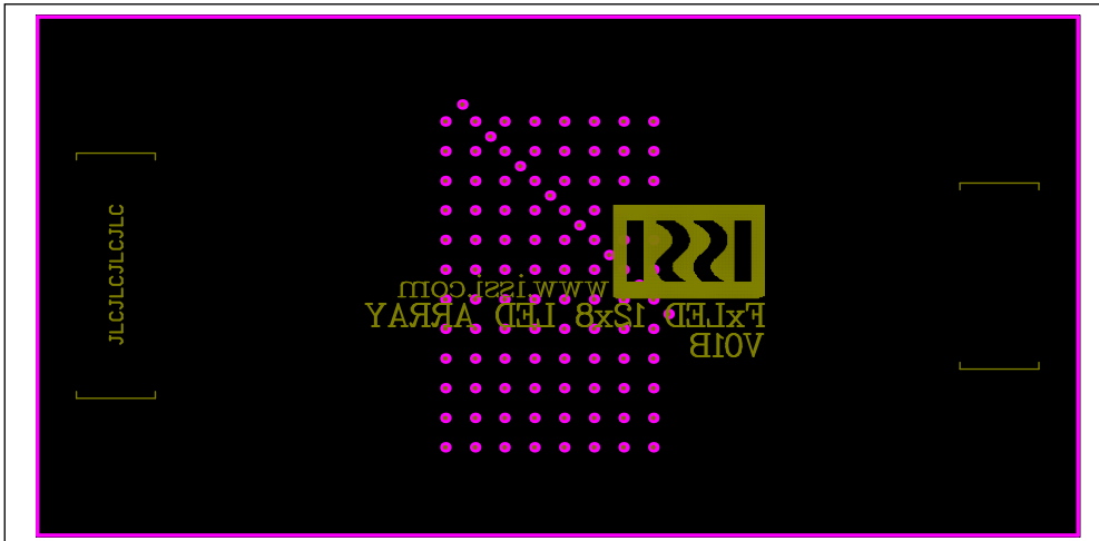
Figure 10: LED Board Component Placement Guide - Bottom Layer
