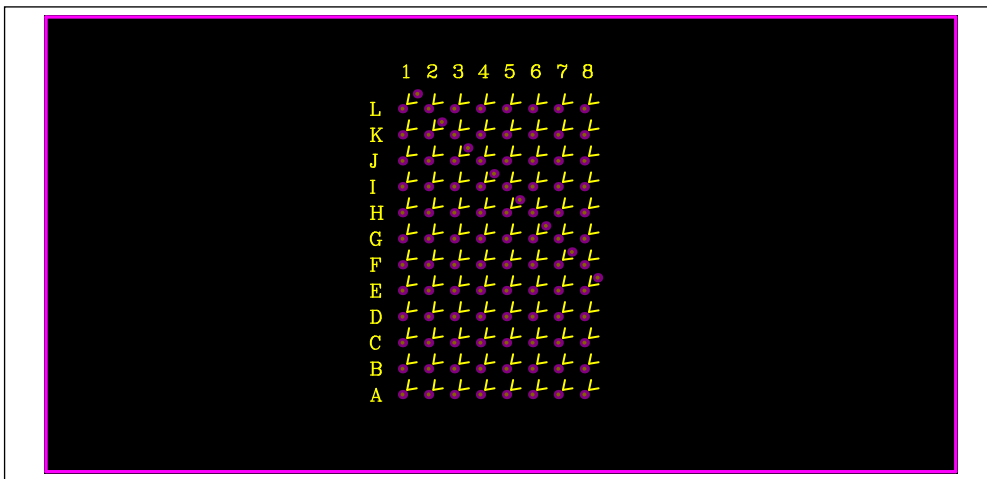
Figure 8: LED Board Component Placement Guide - Top Layer
