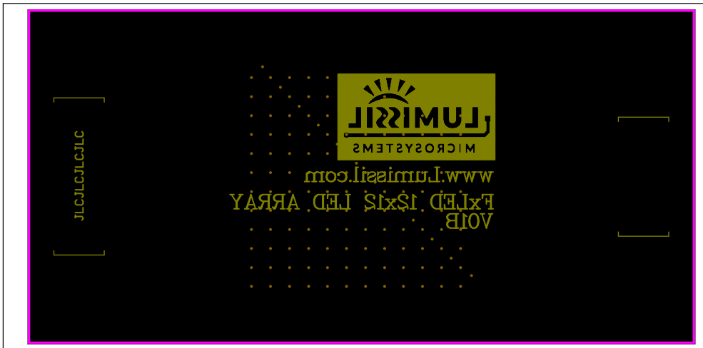
Figure 10: LED Board Component Placement Guide - Bottom Layer
