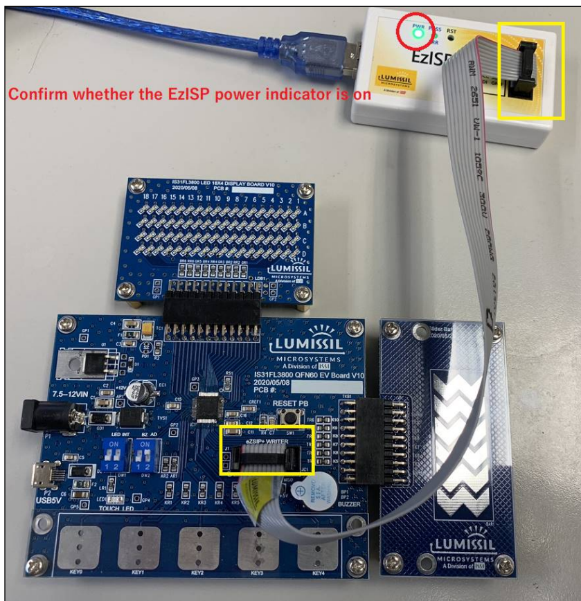
Figure 11: Connection of IS31FL3800 evaluation board and EzISP board
