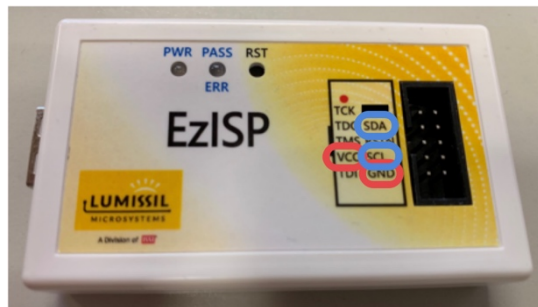
Figure 47: Pin configuration on EzISP board
