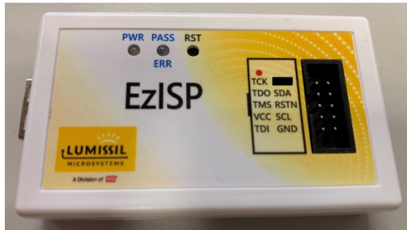
Figure 6: Photo of EzISP Board
