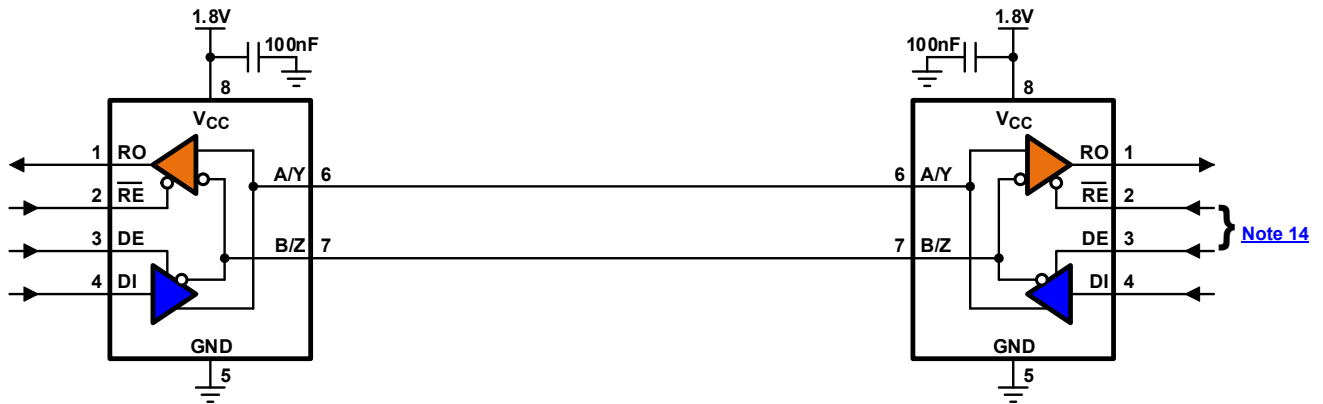
FIGURE 3. HALF DUPLEX NETWORK USING ISL32603E
