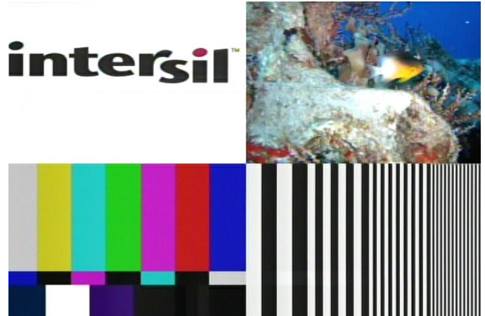
FIGURE 18. TEST PATTERN IMAGE AFTER 5200 FEET OF CAT 5 WITH ISL59605
