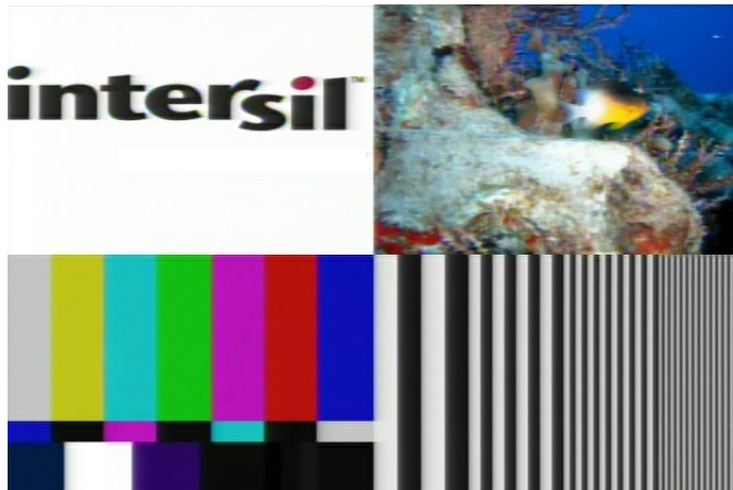
FIGURE 1. TEST PATTERN IMAGE AFTER 1000 FEET OF UNCOMPENSATED CAT 5
