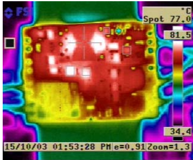
FIGURE 15. THERMAL IMAGE: 48V INPUT, 300LFM AIR FLOW
