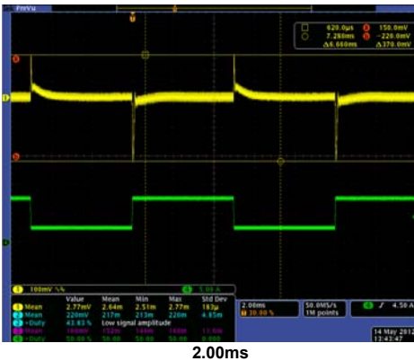
FIGURE 13. 36V INPUT, CH1: OUTPUT VOLTAGE, CH4: LOAD CURRENT
