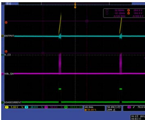
FIGURE 36. OVERCURRENT PROTECTION, CH1: OUTPUT VOLTAGE, CH2: VOLTAGE ON C3, CH3: Vds OF Q4_SR, CH4: LOAD CURRENT
