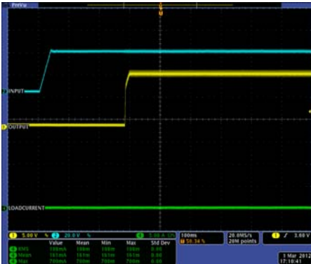
FIGURE 16. NO LOAD START-UP, CH1: OUTPUT VOLTAGE, CH2: INPUT VOLTAGE, CH4: LOAD CURRENT
