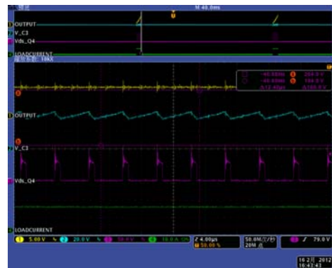
FIGURE 37. ZOOM IN, CH1: OUTPUT VOLTAGE, CH2: VOLTAGE ON C3, CH3: Vds OF Q4_SR, CH4: LOAD CURRENT
