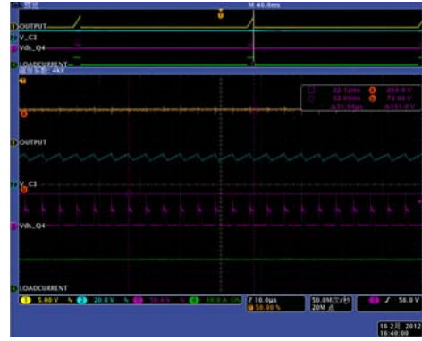
FIGURE 33. ZOOM IN, CH1: OUTPUT VOLTAGE, CH2: VOLTAGE ON C3, CH3: Vds OF Q4_SR, CH4: LOAD CURRENT
