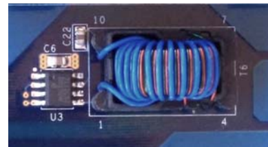
FIGURE 9. PULSE TRANSFORMER AND DRIVER
