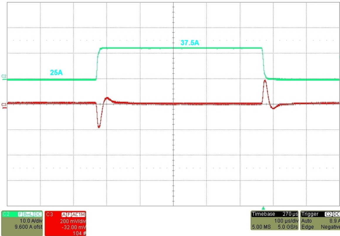
FIGURE 24. STEP LOAD: 25A TO 37.5A (12.5A DELTA)
