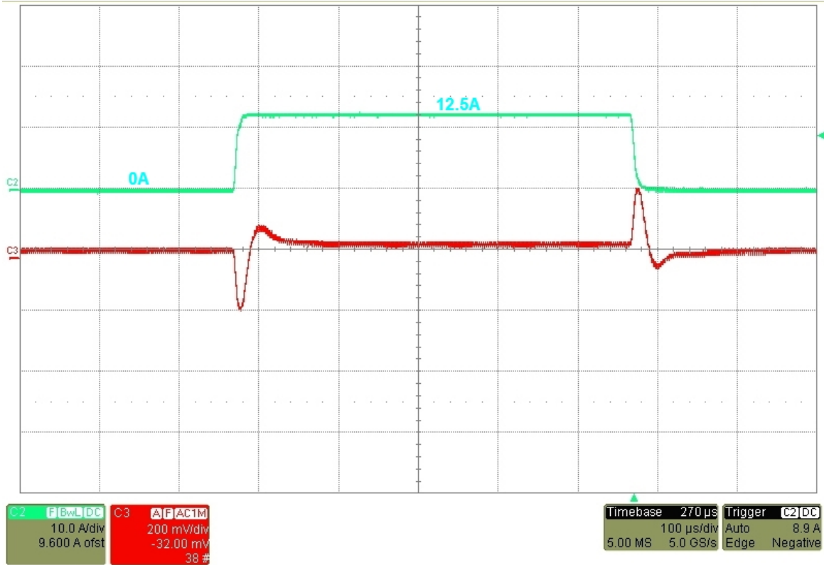
FIGURE 23. STEP LOAD: 0A TO 12.5A (12.5A DELTA)
