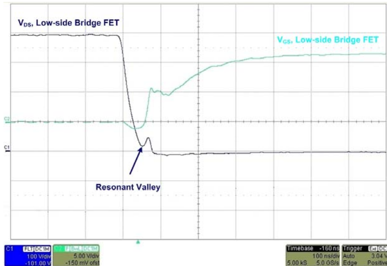
FIGURE 21. RESONANT SWITCHING WITH 100% (50A) LOAD
