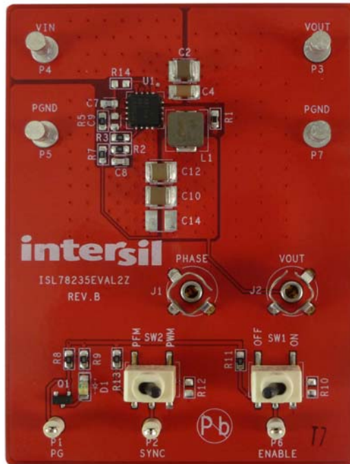
FIGURE 2. ISL78235EVAL2Z TOP SIDE
