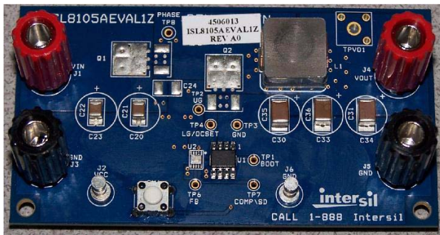
FIGURE 1. ISL8105AEVAL1Z EVALUATION BOARD
