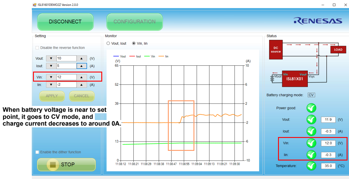
Figure 13. Fully Charging Information in GUI
