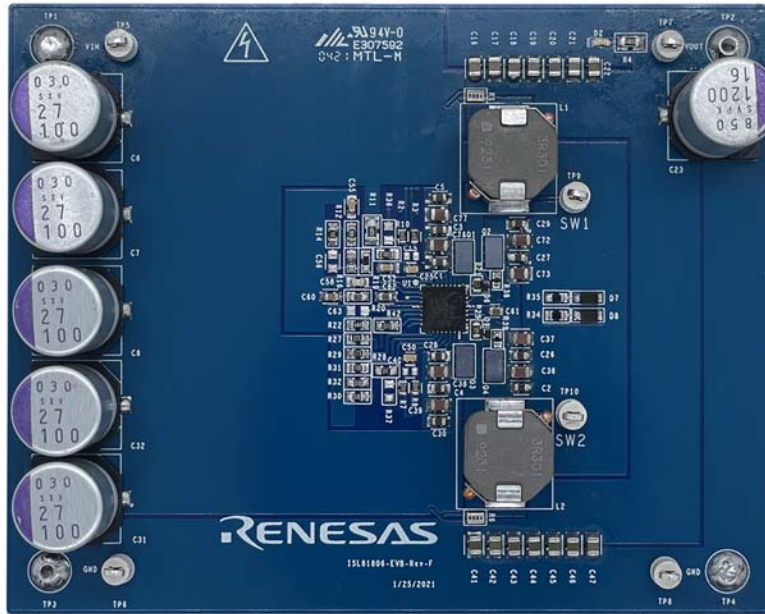
Figure 4. ISL81806EVAL1Z Evaluation Board, Top View
