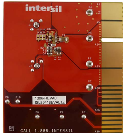
FIGURE 7. BACK OF EVALUATION BOARD ISL85418EVAL1Z
