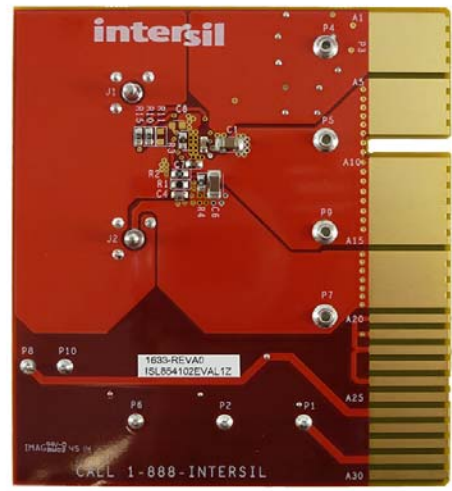
FIGURE 5. BACK OF EVALUATION BOARD ISL854102EVAL1Z
