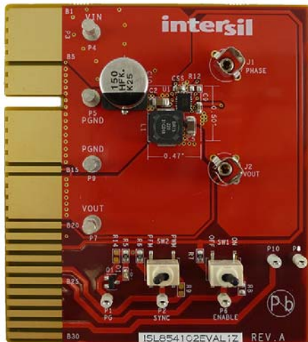
FIGURE 4. FRONT OF EVALUATION BOARD ISL854102EVAL1Z
