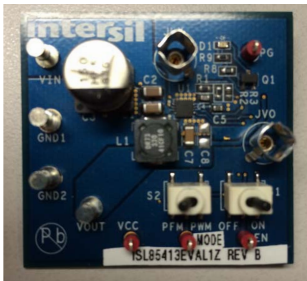
FIGURE 1. FRONT OF EVALUATION BOARD ISL85413EVAL1Z
