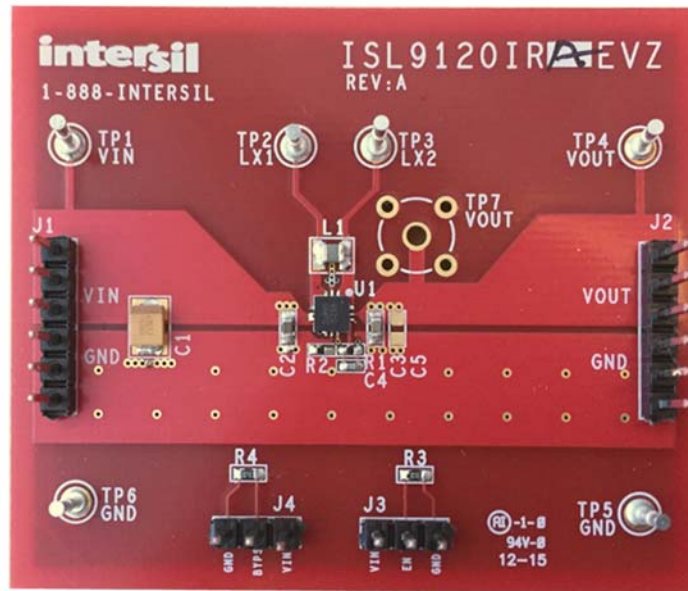
FIGURE 4. ISL9120IRA-EVZ EVALUATION BOARD
