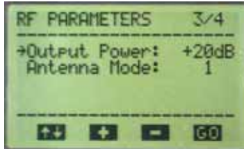
Figure 18. Screen 3: RF Parameters (Antenna Diversity Card Fitted)
