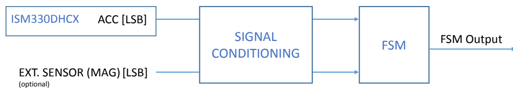
Figure 2. State machine in the ISM330DHCX
