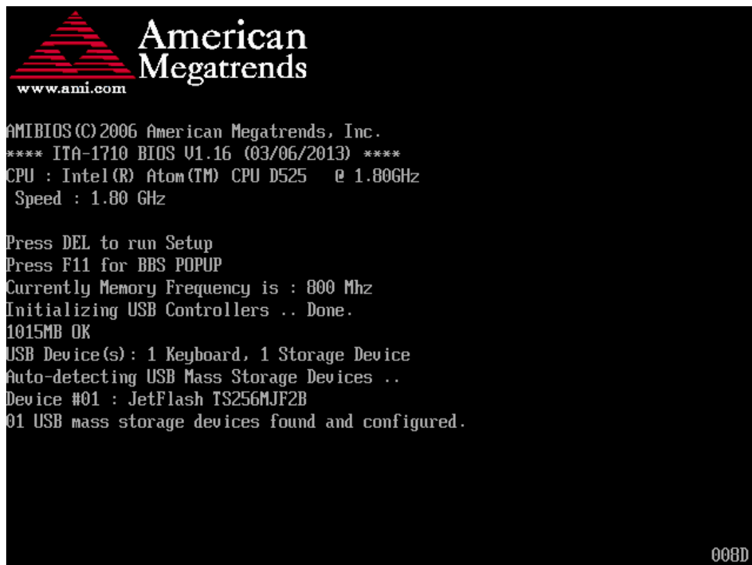
Figure 4.2: Press <DEL> to Enter Setup
