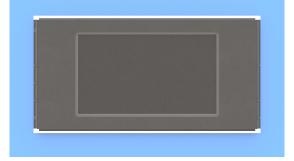
A hole the size of the rear of the module, with enough clearance for the electronics, is formed in the product, and the IoD-SM sits in the hole with the surface mount pads being soldered from the front, and its electronics accessed through the hole.
