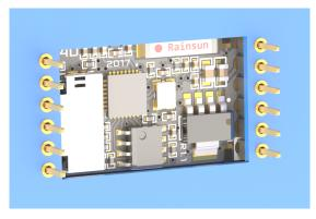
The IoD-09SM features surface-mount castellated pads and is designed to be soldered in place onto a host PCB. This module can be mounted on a PCB in 2 main ways.
