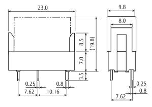
PC Board Mouting Hole Layout (BOTTOM VIEW)
