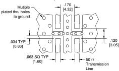
Dimensions are in Inches [Millimeters] JP506S Mounting Footprint
