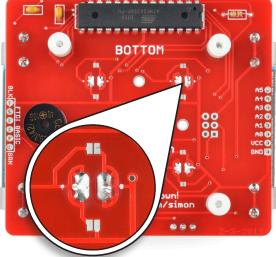
Using a hobby knife, cut both traces directly over the white dots.
