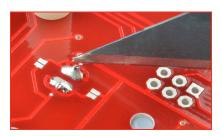
Using a soldering iron, close both jumpers.
