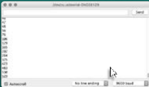
Serial Monitor printout and baud-rate menu.
