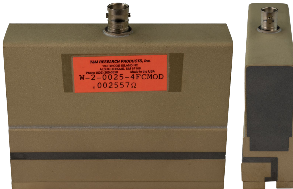
FIGURE 5: T&M RESEARCH W-2-0025-4FC 2.5 m \Omega CVR
