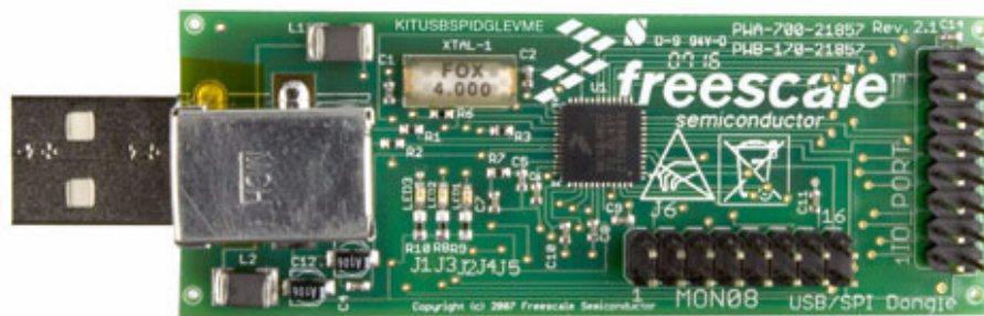
Figure 6. KITUSBSPIDGLEVME Interface Dongle
