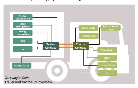
The new 24V Automotive gateway board features two powerful AURIXTM TC397 microcontrollers combined with the RTL9047AA automotive Ethernet switch from Realtek. The two AURIX™TC397 bring the well-known multicore computing performance, flexibility, scalability, integrated safety and security support of the AURIX™ 2<sup>nd</sup> generation
