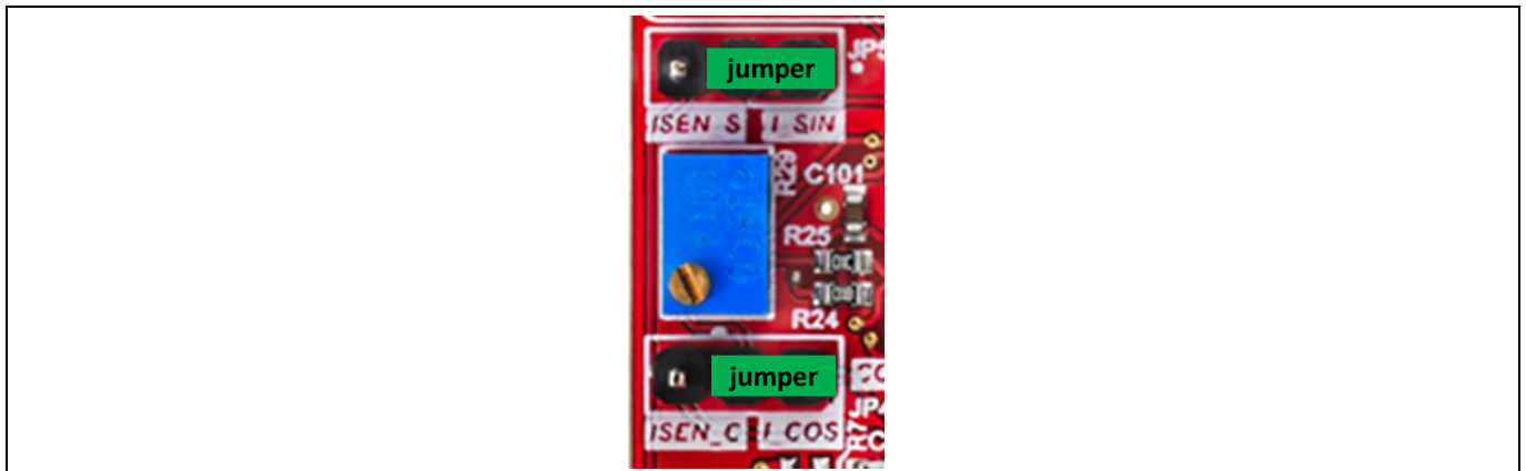
Figure 8 Jumper setting: Connect to I_SIN and I_COS
