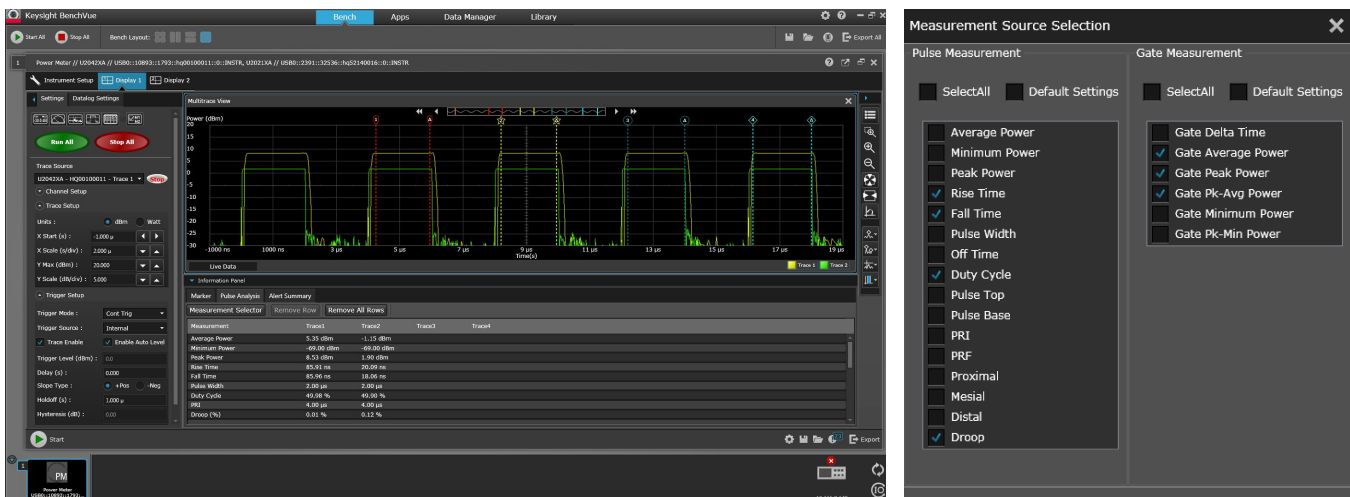
Figure 8. Multi-channel trace display with 4-pairs of gates and automatic pulse parameters measurement (sample screen shot with two X-Series power sensors)
