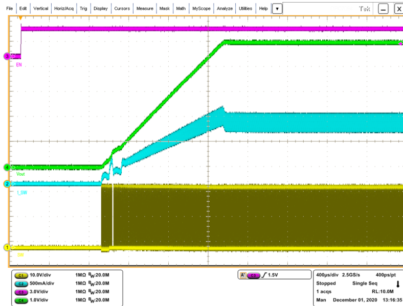
Figure 7. Soft-start phase with I_{OUT} = 1.25\text{ A}
