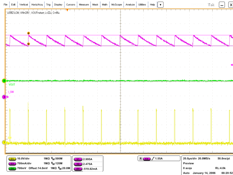
Figure 22. Over current procedure with persistent short circuit between VOUT and GND
