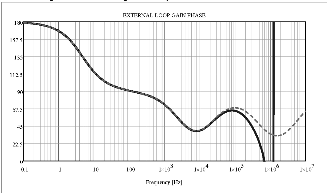
Figure 45. Phase margin Bode's plot of L6985F evaluation board
