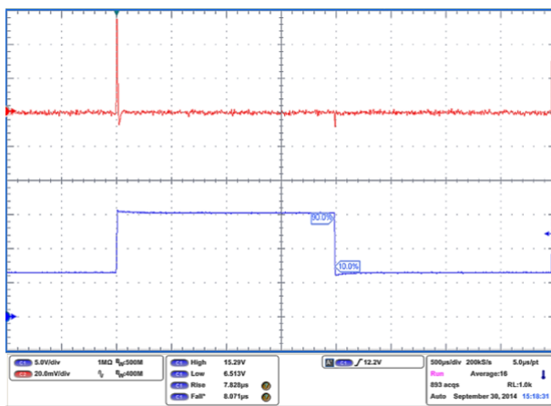
Figure 24. Line transient ( V_{OUT} = 5\text{ V} )
